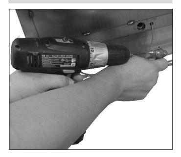
**8. Fasten the New NG Regulator** Fasten on the NG Regulator, with the Female Flare Adapter connecting to the Grills Right Back Side Gas Manifold Male Flare Adapter. Notice Arrow indicating direction of Gas Flow.
