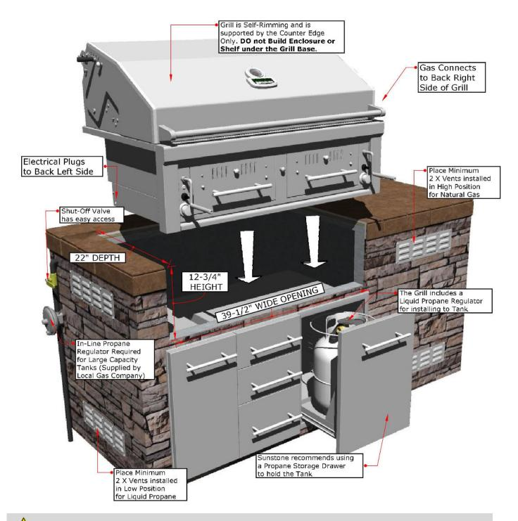
**NOTICE:** All Gas Lines for either Liquid Propane or Natural Gas should be installed by a Licensed Professional <u>ONLY!</u> All Liquid Propane Installation with a Large Capacity Side Yard Tank, requires a Medium Pressure In-Line Regulator to be installed by Licensed Professional. Grill includes LP Regulator for 25 Pound Portable Tank only, if you require grill to use Natural Gas, please call our Technical Support Line and request NG-Conversion Kit for Item No. SUNCHDZ42 at 888-934-9449.
