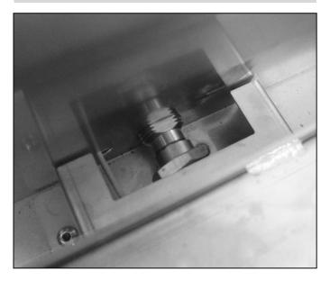
**5. Locate the Flare Adapter in Back** If the Flare Adapter has not been pushed out all the way, do that now by pulling it out, and rotate it slightly revealing the Orifice Hole at tip the Tip of the Flare Adapter Cone.
