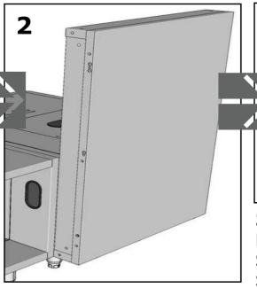
**2.** Hinge the (2) SCC22BPE cabinet panels to the back connecting (2) SCC22PTD Drawer Bases.
