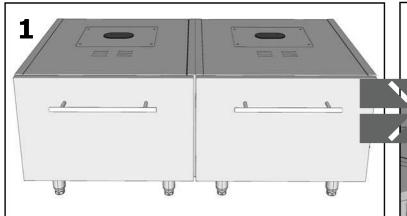
**1.** Fasten on the included (4) Peg-Legs for each of the SCC22PTD Drawer Bases. Lift and Hinge the cabinets together, then secure with connecting bolts. Fasten on both Handles.
