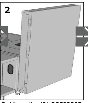
2. Hinge the (2) SCC22BPE cabinet panels to the back connecting (2) SCC22PTD Drawer Bases.
